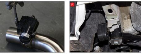
Once happy with fitment of Scorpion Exhaust, fully tighten up all clamps and fixing and plug in the electronic valve motors.
